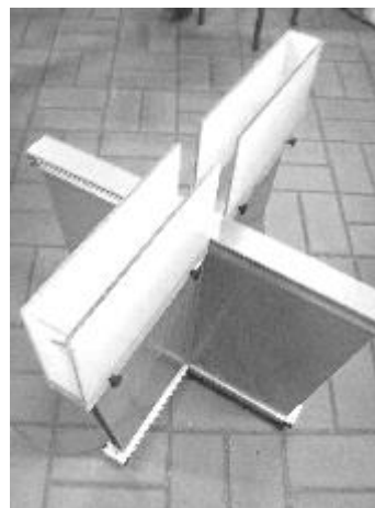
Elevated plus maze apparatus
